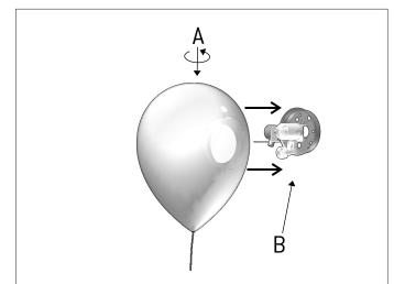
2- Before marking the holes where the mounting bracket (B) will get screwed to the wall, make sure that the piece (D) remains horizontal use a level if needed-Affix the mounting bracket (B) to the wall or the electrical junction box. Insert the electrical wires from the outlet box into the mounting bracket. Connect the electrical wires. Figure 2.
