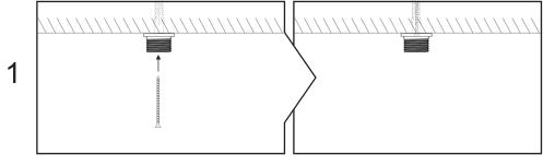
Use the plugs and screws to fasten the top ceiling attachments at the desired location.
