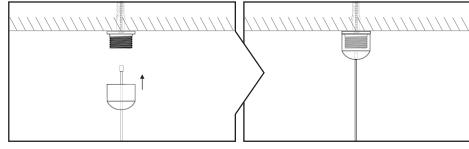
Protrude the wires through the bottom ceiling attachments and screw it on the top attachments.
