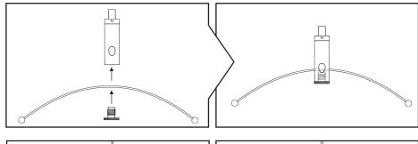
Put the wire bridges inside the slit on the bottom of the grippers and fasten the gripper screws.
