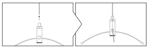
Protrude the wires hanging from the ceiling into the gripper and make sure at least 2cm of the wire is sticking out for safety measures.
