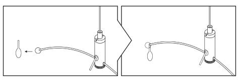
Insert the bridge wire endings into the keyholes of the lamp. Adjust the height and position of the lamp with the wire and grippers.
