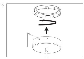
Attach the ceiling plate to the top plate by turning the ceiling plate.
