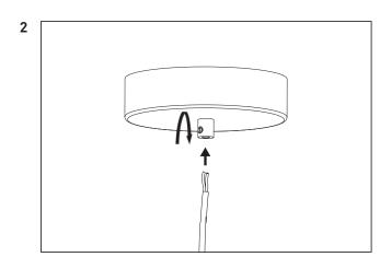
Lead the fabric cable in through the cable relief at the bottom of the ceiling plate. Adjust the cable to the desired length.
