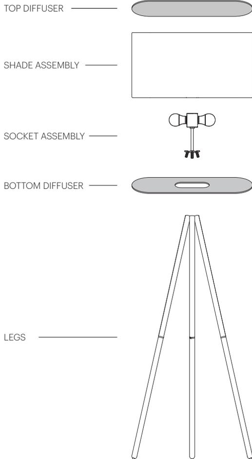
1. ASSEMBLE LEGS (3 LOWER SECTIONS AND 3 UPPER SECTIONS).
