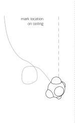
Move pendant into location and mark the location for the swag hook screw on the ceiling.
