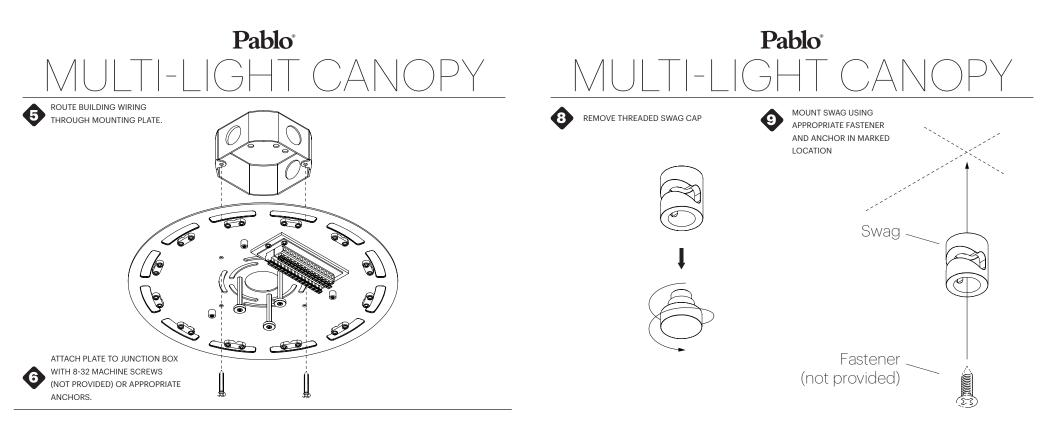
WIRE BUILDING WIRING TO TERMINAL BLOCK.
