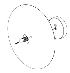
CAREFULLY THREAD GLASS GLOBE ONTO LIGHT ENGINE WITHOUT OVER-TIGHTENING.
