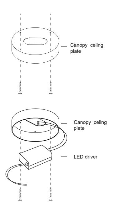
Shut down associated electrical breaker and secure LED driver to top plate of canopy. Then wire LED driver to power source using brown and blue wires.
