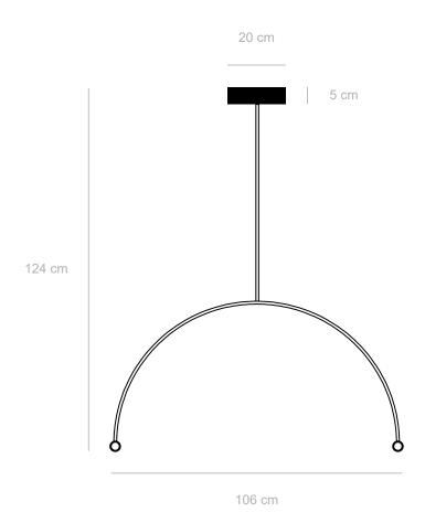
Materials: brass pipe, acrylic tube, LED lights Light: flexible LED strip light, 32W, 24V - UL listed
