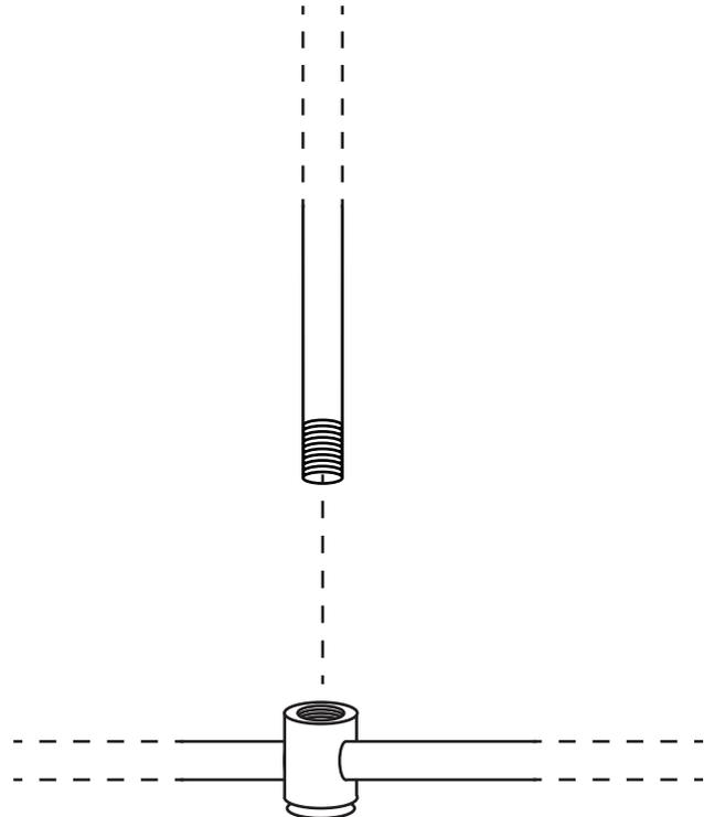
**5** Connect canopy bridge and canopy plate to Tube Pendant stem using the canopy and lock nuts. Make sure to wire through the electricla wires.
