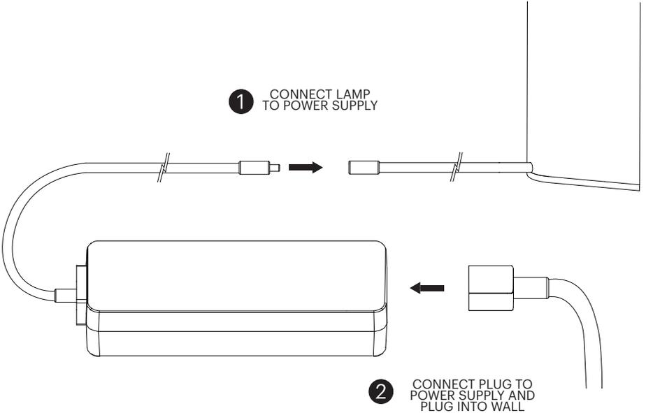
2 CONNECT PLUG TO POWER SUPPLY AND PLUG INTO WALL
