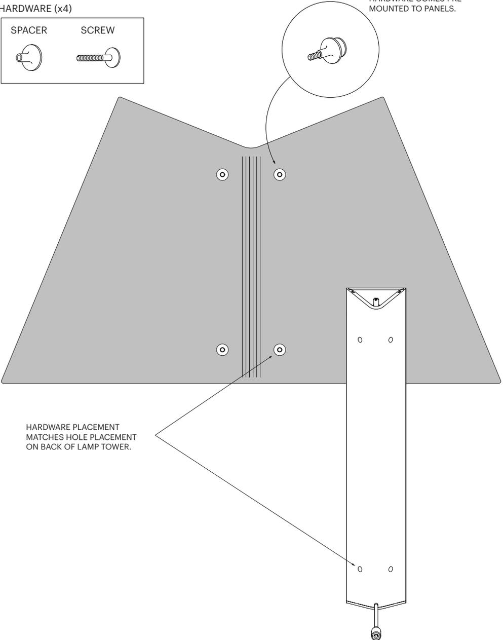
HARDWARE PLACEMENT MATCHES HOLE PLACEMENT ON BACK OF LAMP TOWER.
