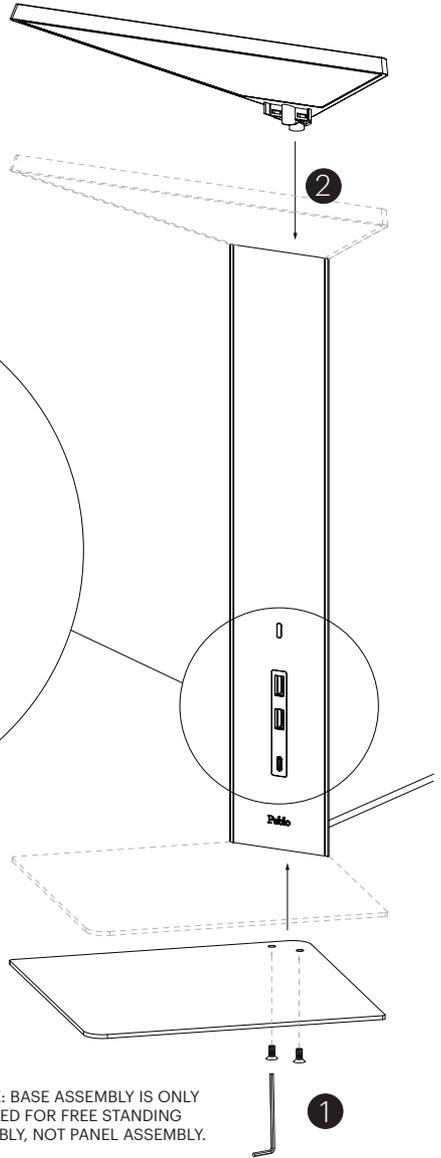
NOTE: BASE ASSEMBLY IS ONLY NEEDED FOR FREE STANDING ASSEMBLY, NOT PANEL ASSEMBLY.
