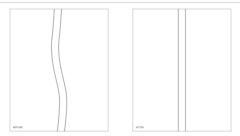
After installation, if the rope appears wavy and does not hang straight, leave the fixture turned on for an hour or so to allow the inner tubing to warm up and soften.
