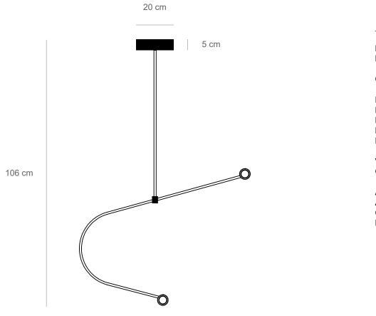
Materials: brass pipe, acrylic tube, LED lights Light: flexible LED strip light, 32W, 24V - UL listed
