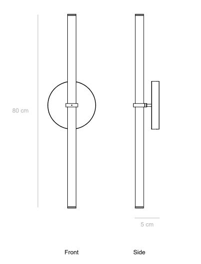
Materials: brass pipe, acrylic tube, LED lights Light: flexible LED strip light, 16W, 24V - UL listed
