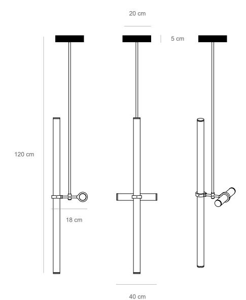
Materials: brass pipe, acrylic tube, LED lights Light: flexible LED strip light, 20W, 24V - UL listed
