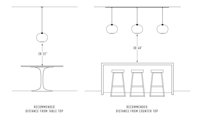
The standard 4' length that comes supplied with your Niche pendant should work for most installations. Your electrician can easily adjust the height up or down before installing so you can get it just right.
