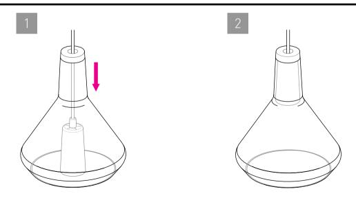
Feed the Drop Cap pendant cable through the plastic fitting at the top of Drop Top shade until the Drop Top shade is resting on the Drop Cap Pendant.
