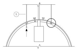
Slide both ends of the steel strings (5) into the Reutlinger cable grippers (8) from the bottom of the canopy (9) and adjust the final height of the fixture.
