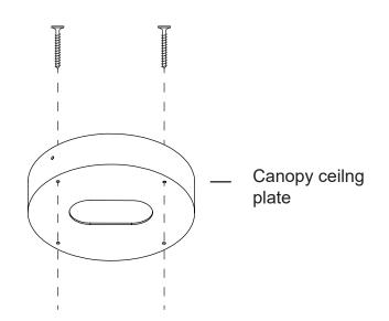
Shut down associated electrical breaker and secure LED driver to top plate of canopy. Then wire LED driver to power source using brown and blue wires.
