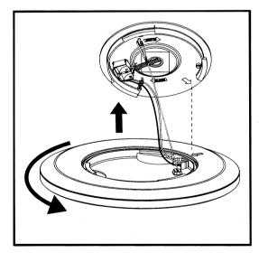
Place LED lamp as shown with marked arrows. Once LED lamp is lifted in place, turn clockwise to lock it in position. Make sure LED lamp locks to it's place.
