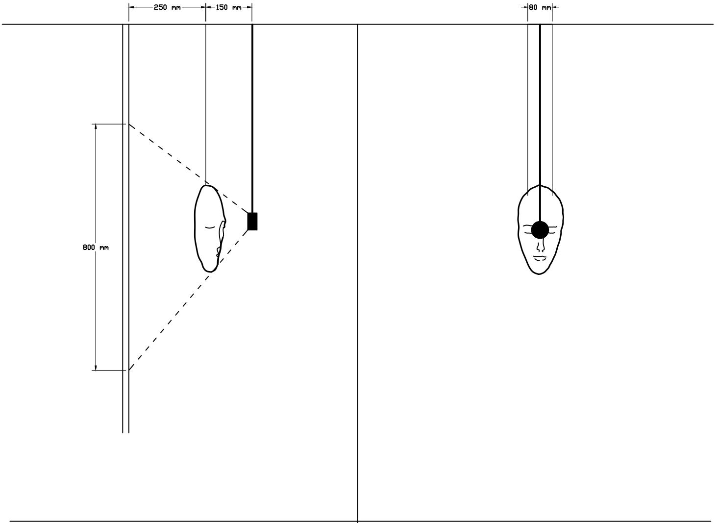
If the installation is separated from the wall by 9,8 in, the projection is 31,4 in.
