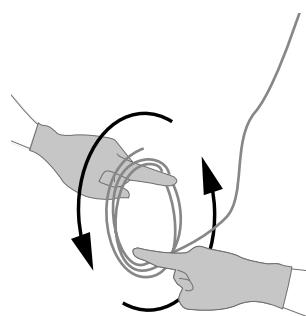
**EN** To avoid kinks, uncoil the sculptural cable in a spool-like manner. Allow the cable to uncoil completely before installing.
