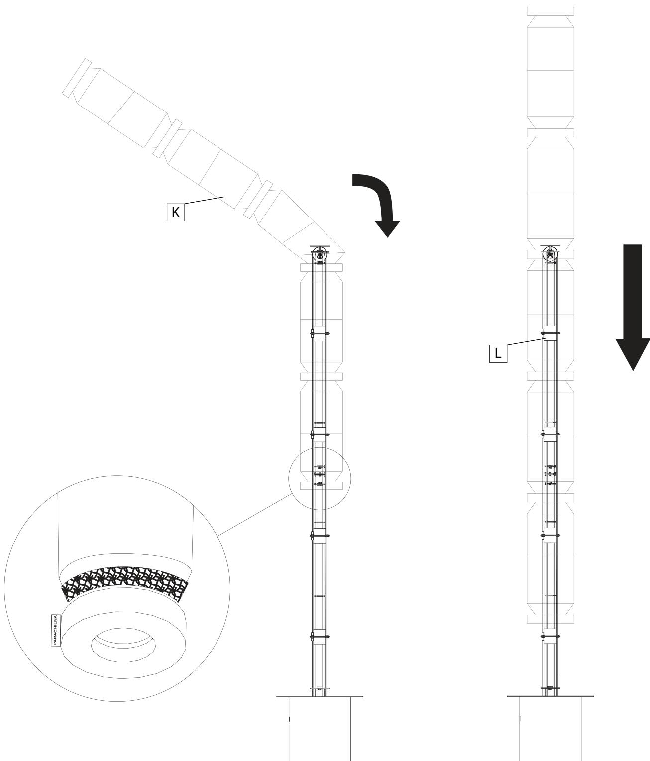
**EN** Place shade (K) carefully on to the light structure. Note that there is a specific way to place the shade. Ensure that the end with the black tape goes over first. Once the correct end has been identified, remove the tape. When placing the shade, it is necessary to stretch the fabric to fit over the components (N), do it without fear.
