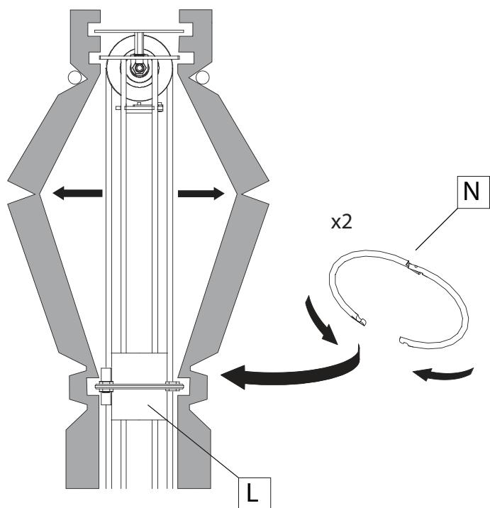
**EN** 10.1 Stretch out the shade to raise it and be able to align the double exterior notches with the plastic part (L).
