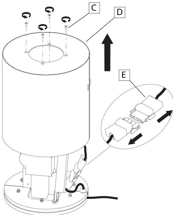
**EN** Unscrew the screws (C) and remove the cylinder (D) that covers the body of the base. Disconnect the connect (E).
