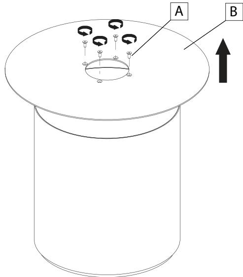
**EN** Remove the screws (A) to remove the disc (B).
