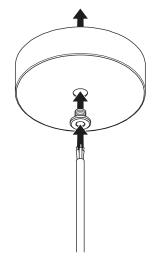
Mount the back plate onto standard 4" octagonal junction box. If you do not have one in the desired position, get your electrician to install one. Fixings not supplied. Suitable junction box bolts should be used.s
