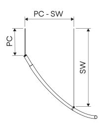
Curved rods B and C have variable suspension options. By turning the ring, you can rotate the rod in different ways in space. The principle of rotation is shown in the figure below. We are looking directly at the suspended rod so that the power cable and steel wire are aligned behind each other and the mounting is closer to us.
